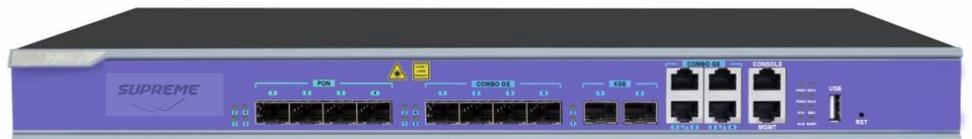
GPON OLT FD1604S-B1 completely meet relative standard of ITU G.984.x and FSAN, which is 1U rack-mounted device with 1 USB interface, 4 uplink GE ports, 4 uplink SFP ports, 2\*10GE uplink ports and 4 GPON ports. Each GPON port supports the splitting ratio of 1:128, The GPON system supports up to 512 terminal connections.
