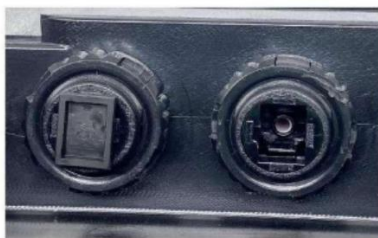
Internal side: Standard SC coupler
